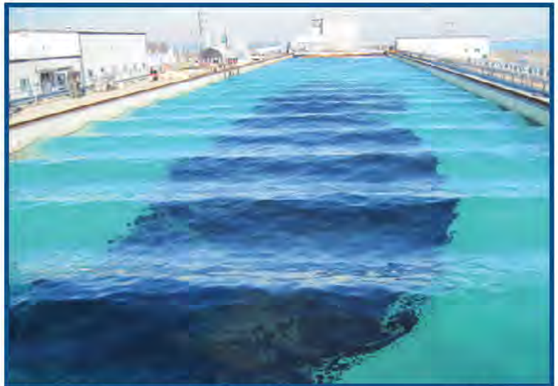
Ohmsett Wave Tank: The VIMS researchers compared the performance of acoustic and optical instruments using this oil slick in the Ohmsett wave tank. Photo by Paul Panetta.
