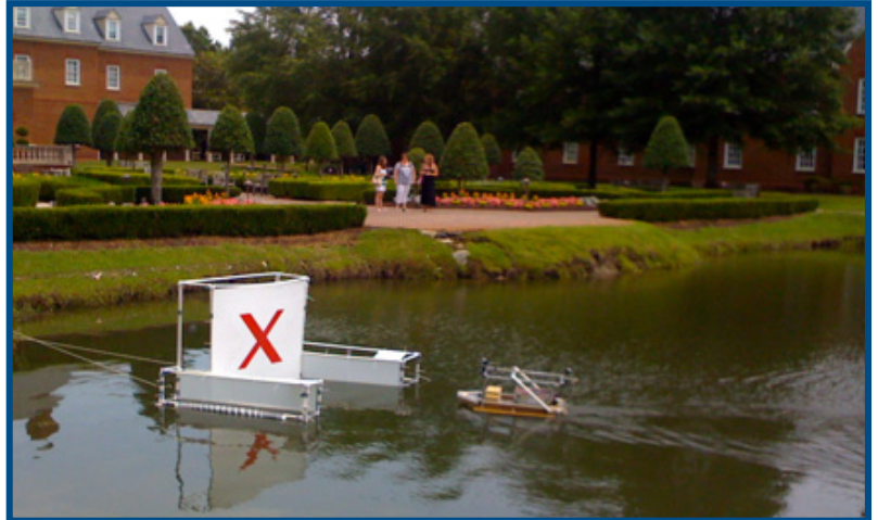
An Autonomous Surface Vehicle (robotic boat) uses computer vision to dock with a target in the 2009 competition.
